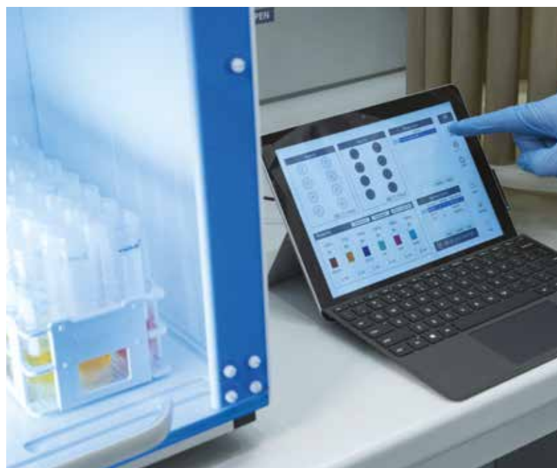
Automatic pre-dilution in 50-mL ICP autosampler vials
