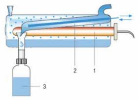
Figure 2: duoPUR acid purification system.
